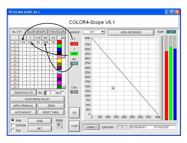
Now press the SEND button again to inform the sensor about the taught color. Then activate the GO mode again. When the sensor recognizes a line vector (color), the responding line number is visualized in C-No: at the software user interface. The value 255 means that none of the taught colors has been recognized.
